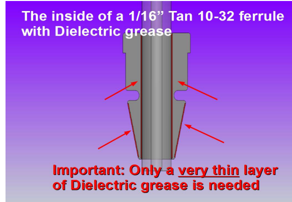
Figure 1B: Applying Dielectric Grease to the Tan Ferrule.
