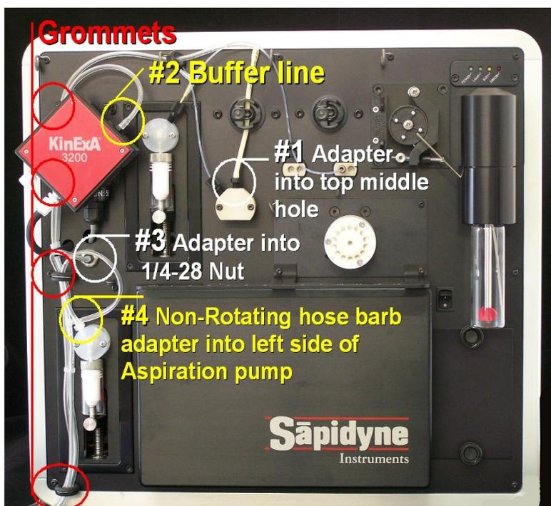
Figure 1: Buffer Waste Connection routing diagram.
