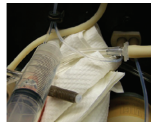
Figure 5. Pushing dH 2 O through the solenoid valve.
