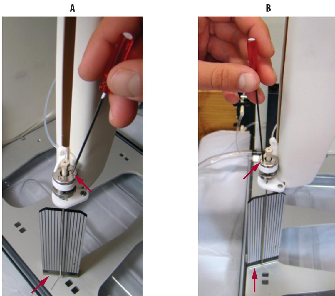
**Figure 2.** Place the alignment tool on one of the drawn lines on the Autosampler plate with the position facing away from the Autosampler (**A**) and then position facing the particle reservoirs (**B**).
